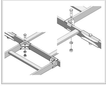
• Includes 4 brackets, 2 nuts and 2 bolts to splice 1 section of ladder perpendicularly to another
