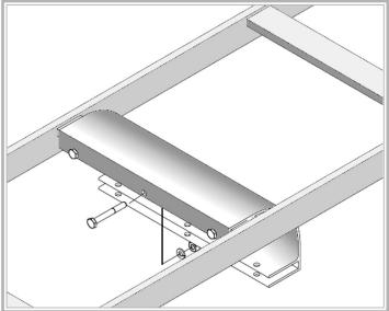
• Includes 1 radius controlled drop, 6 bolts and 3 nuts
