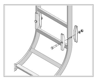
• Includes 4 brackets, 2 nuts and 2 bolts to splice 1 section of ladder as an extension of another
